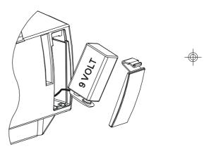
4.) Push the battery back into the battery compartment and replace the battery door.
